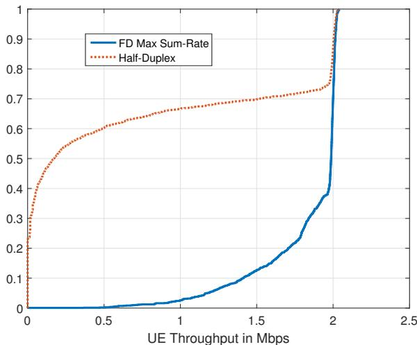
Figure 6. FD gain in UE throughput
