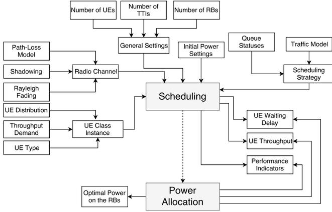
Figure 1. Schematic block diagram of the simulator
