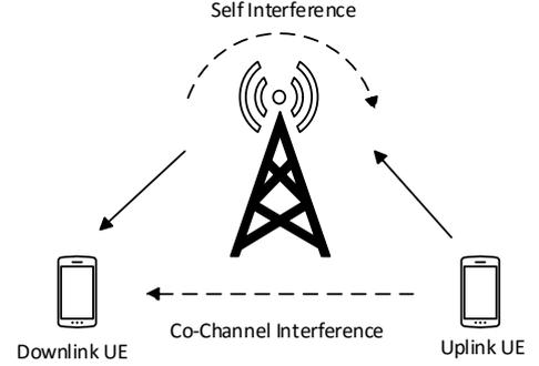
Figure 2. FD-OFDMA network and interferences
